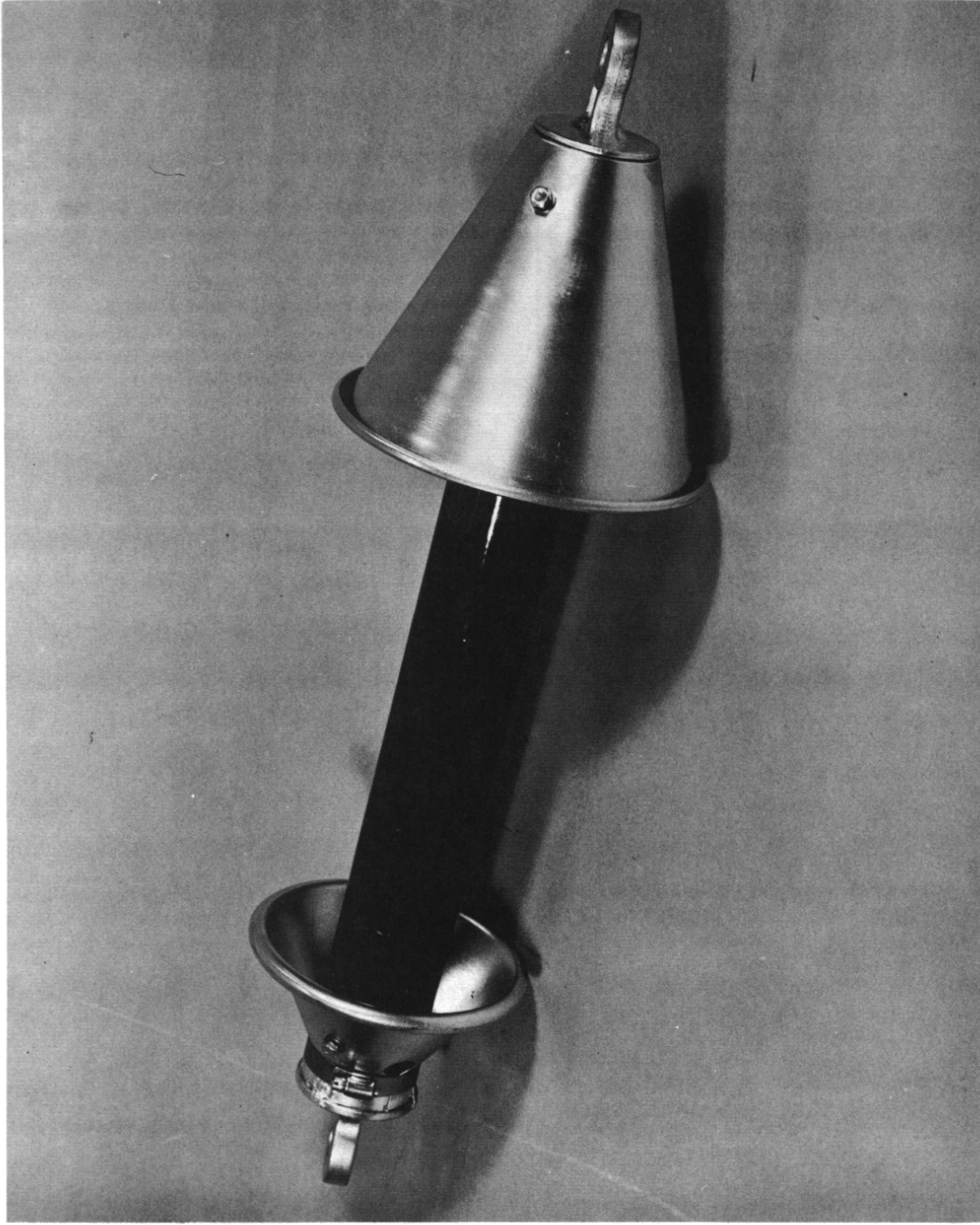
FIGURE 9. AUSTIN SAFETY CORE, OIL FILLED, GUY STRAIN INSULATOR TYPE A-4006 - WORKING LOAD 10, 500 POUNDS.
